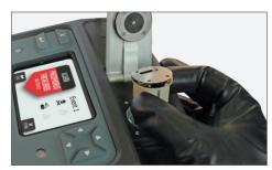
Patented microscale ion trap technology enables operation without the need for extreme vacuum or additional gas supply.
